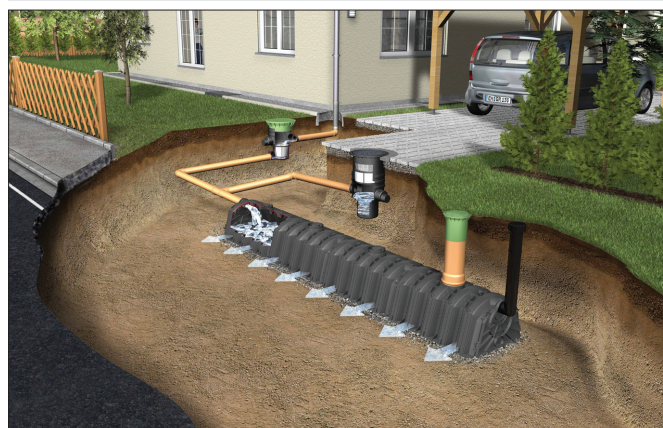
Figure 3 Typical air vent connections and pipework
